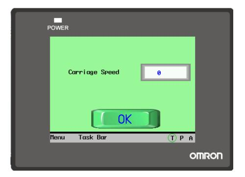
Use this screen to adjust the speed at which the carriage moves to the home position and/or to the right or left when the jog buttons are pressed.
