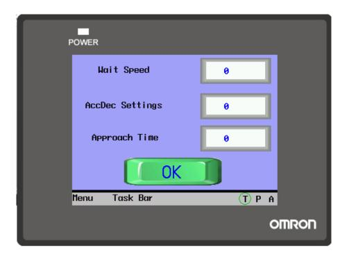
To avoid damage to the Teflon bands, the sealer starts rotating when the welder is switched off. Use this screen to adjust the speed of the sealer in the open position and its acceleration if desired.
